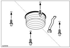
■ Drill four <sup>3</sup>/<sub>16</sub>" (5 mm) holes in the ceiling.
